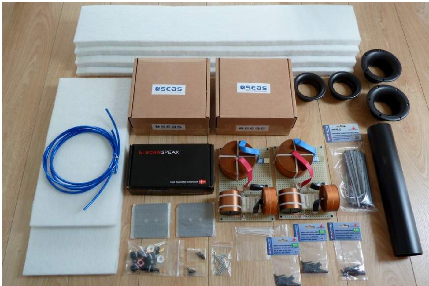
Contents of the Humble Homemade HiFi DIY loudspeaker kit Plutone with the standard crossovers.
